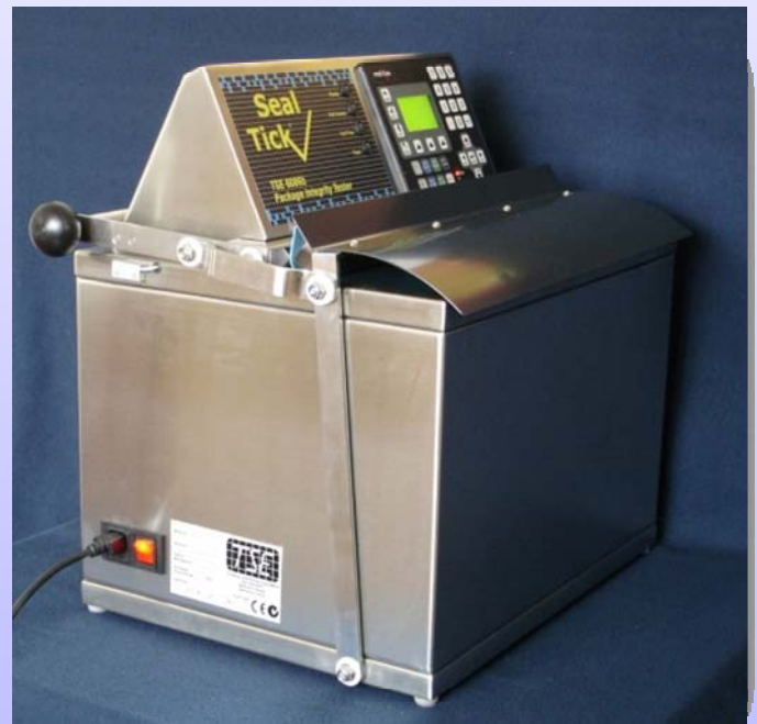
Seal Tick in operation position, closing the handle manually begins the test cycle.
